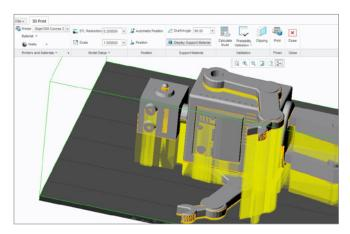
Position the model on the print tray and view the required supporting material in PTC Creo.
