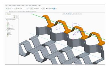
Create sheetmetal geometry using functionality to automatically apply bend relief, create sheetmetal rips, bend coplanar geometry, and more.
